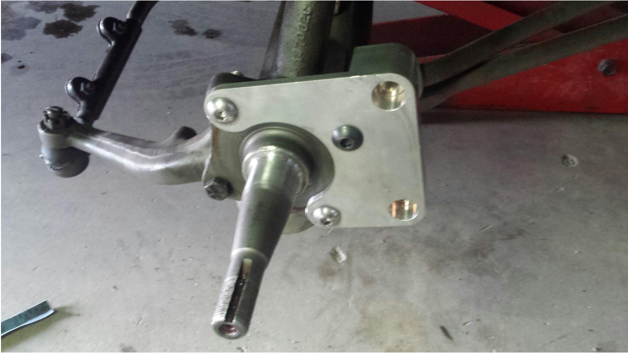
Installation of front adapter bracket. Left side shown.
