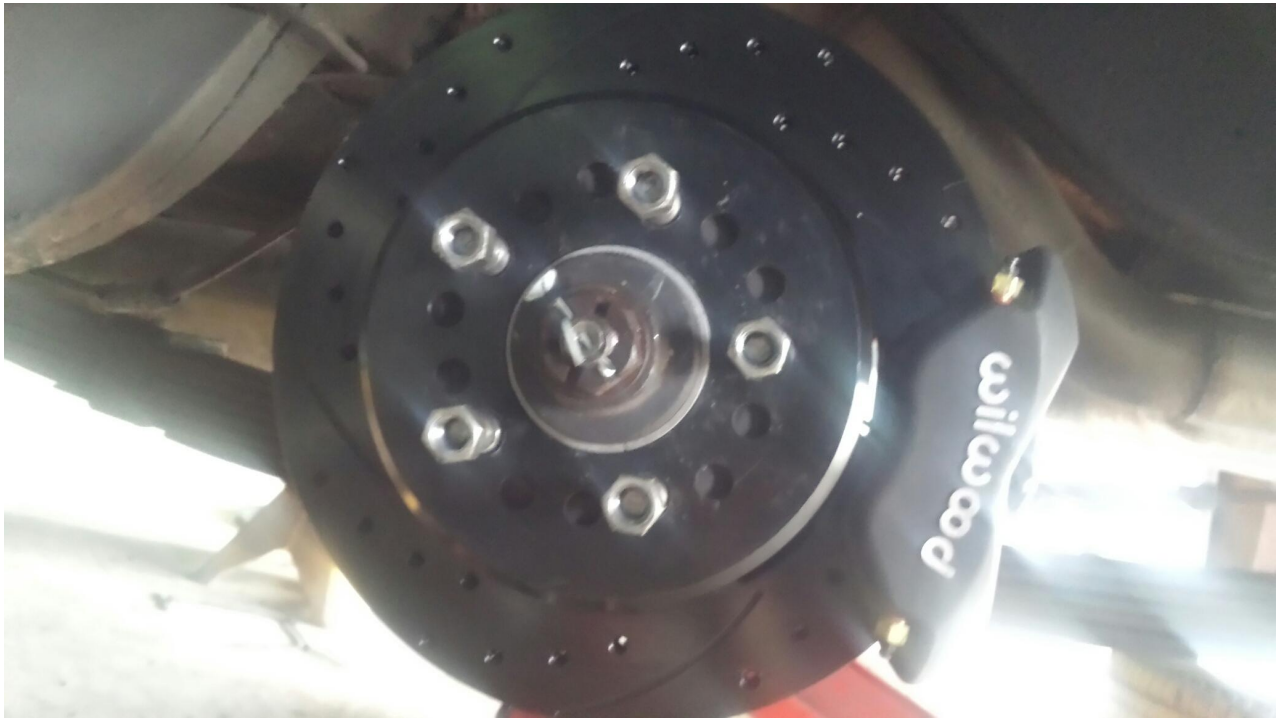
Completed installation of Wilwood rear disc brake conversion. Note the hub has been attached to the axle using cotter pin & nut with keyway.
