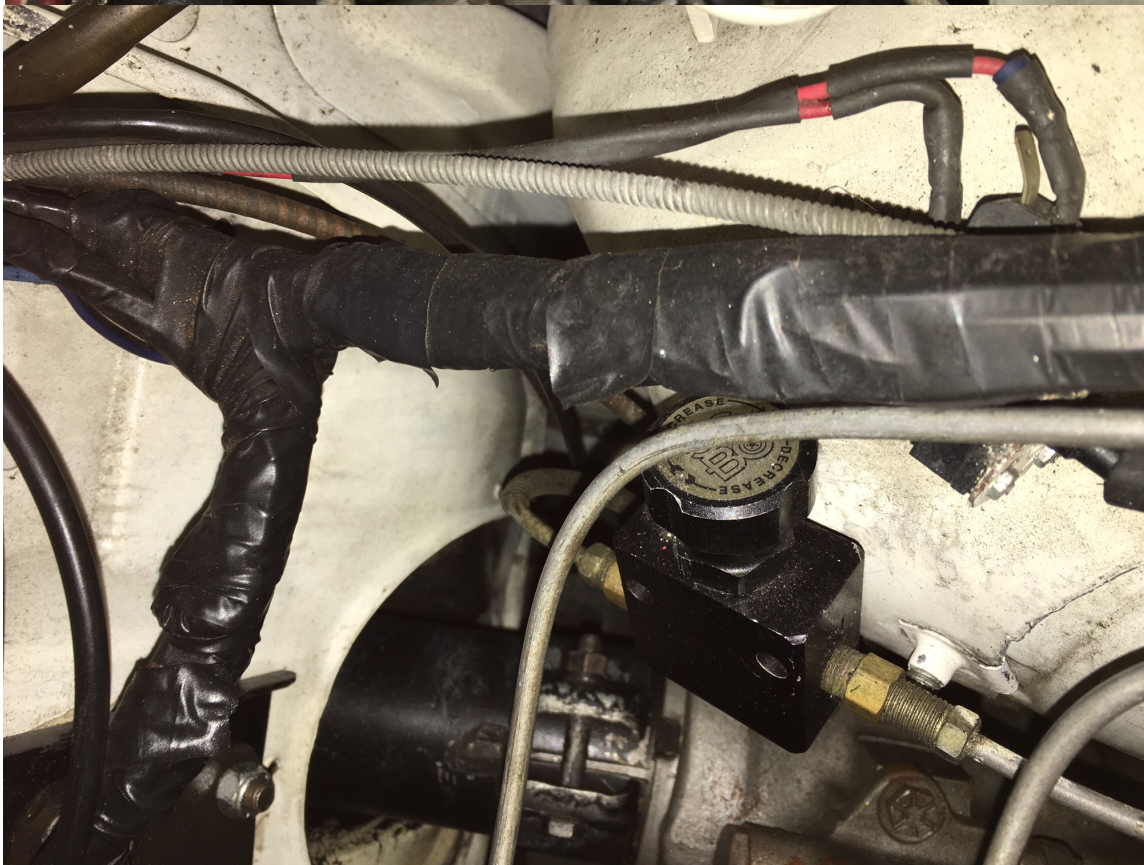
Above: new master cylinder. Below: Proportioning Valve
