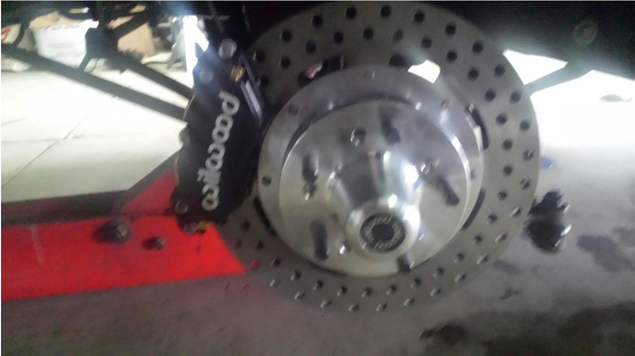
Completed installation of Magnum Force/Wilwood disc brake conversion. Right side shown.
